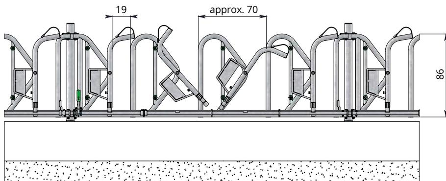
Sectional view installed feed front
