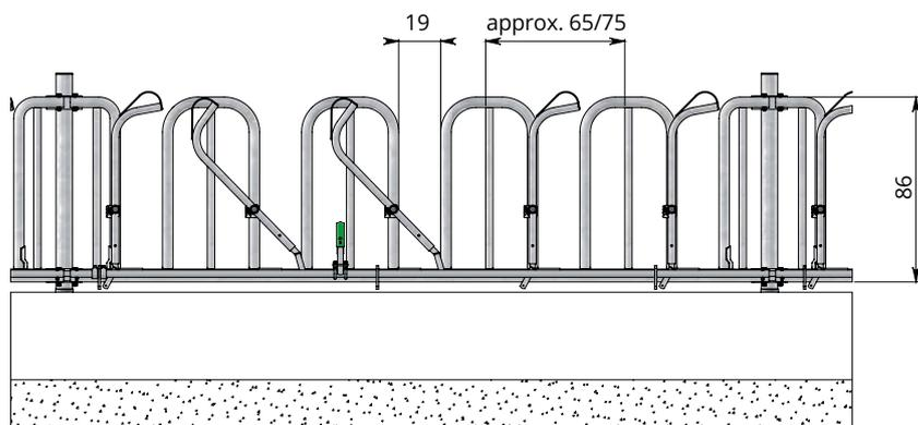
Sectional view installed feed front
