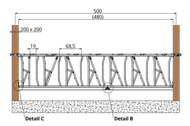
On this page we present two solutions for the installation of Highline feed fronts to support columns measuring 5.00 m centre-to-centre. The choice was made to attach it to HEA180 posts or to square (wooden) columns 200 mm.
