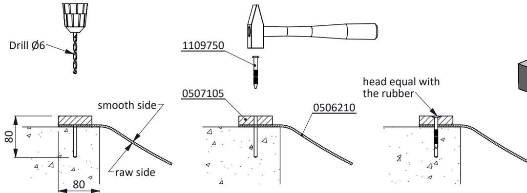
**Attention: On both ends of the row of stalls mount the rubber strip 10 cm of the ends; this to leave room for the aluminium mounting strips which have to be mounted later.**
