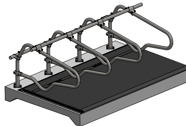
**Attention: On both ends of the row of stalls mount the rubber strip 10 cm of the ends; this to leave room for the aluminium mounting strips which have to be mounted later.**
